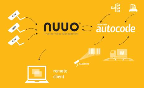
Autocode is a video analytics module for Mainconsole (NUUO) surveillance systems, that provides automatic car number plate recognition (ANPR), railway wagon numbers and container code recognition.
